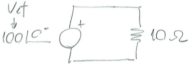
$$\bar{I} = \frac{\bar{V}}{\bar{Z}} = \frac{\bar{V}}{R + j0} = \frac{V_{eff} \angle \varphi}{R \angle 0^\circ} = \underbrace{\left(\frac{V_{eff}}{R}\right)}_{I_{eff}} \angle \varphi$$
